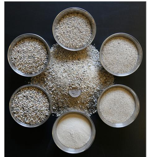
A visual breakdown of an ideal grade-blend for effective lime plaster sand. Blended grades, especially angular manufactured sands, create a very efficient void structure, which allows for better workability, better mechanical bonding, and proper vapor exchange (breathability) in the cured plaster.
